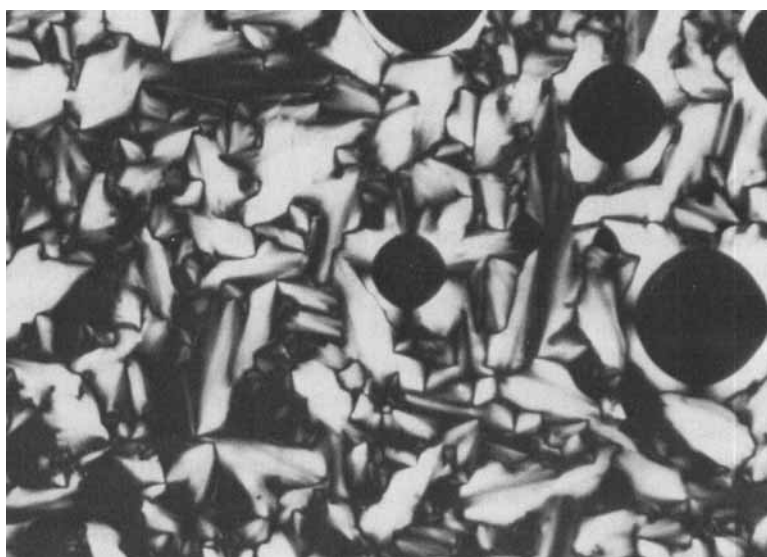
FIGURE 4 Texture of \text{PbC}_{10} smectic phase at 382.5K; mag. \times 40
